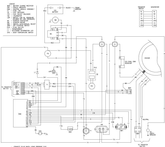
$\star$  connect plug when using propane fuel disconnect when using natural gas
